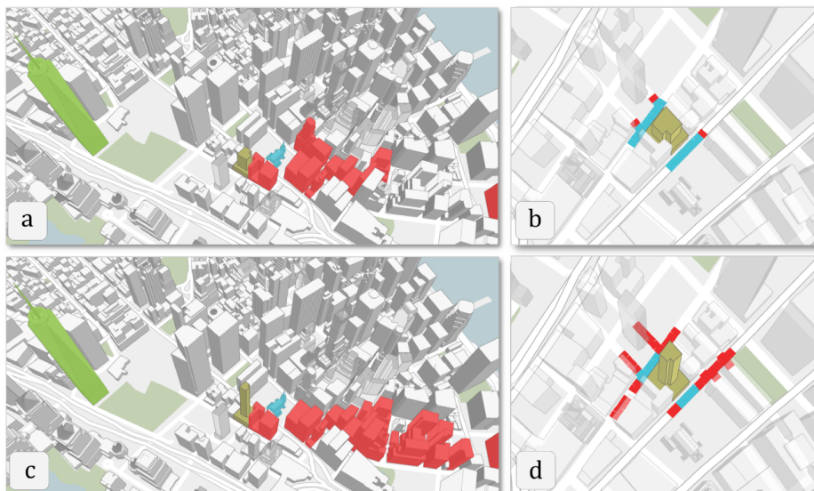
Figure 7: Understanding the impact of different building designs. The view (a) and sky exposure (b) impact when using a 80 \times 120 floor plate vs. the impact when using a 65 \times 65 floor plate (c & d) for the proposed buildings.
