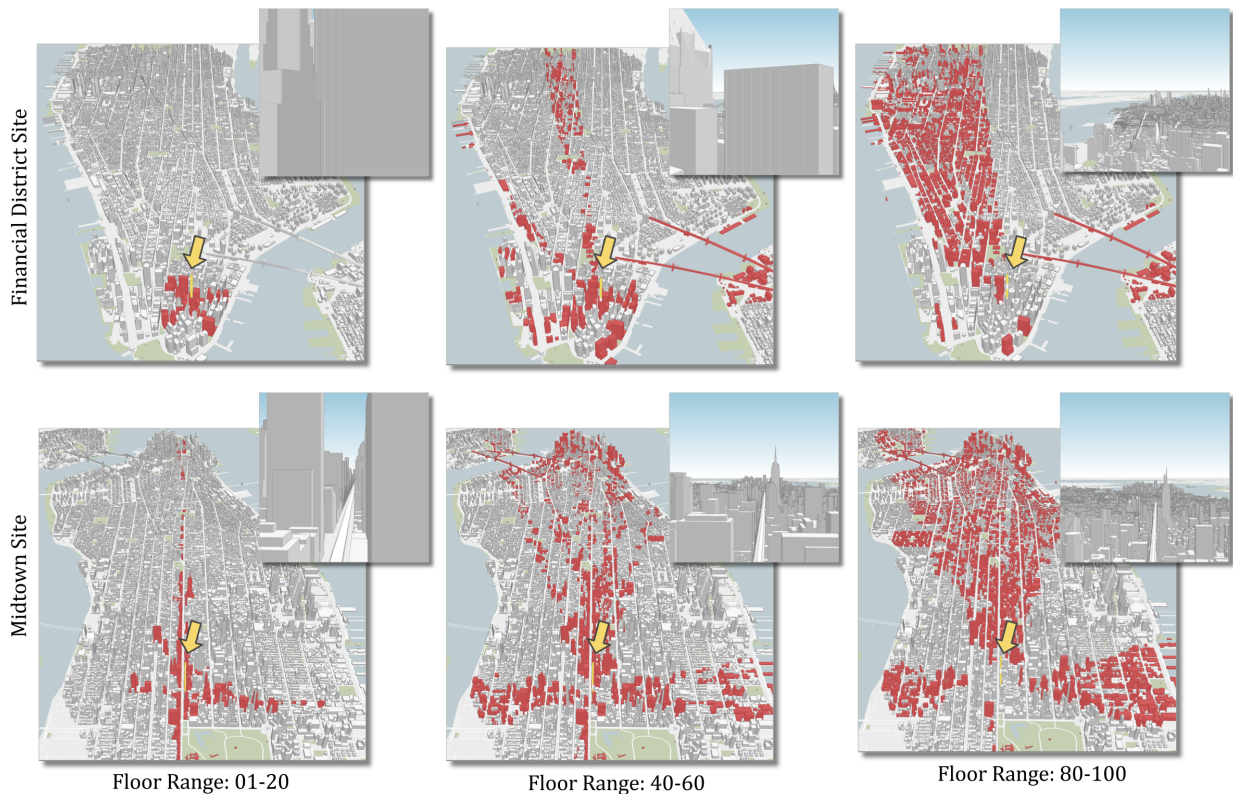
Figure 10: The views obtainable from different height zones (20 floors each) from the two sites in Financial district and Midtown. The buildings highlighted in red indicate the reach from these zones. The inset shows the typical view from a representative window.
